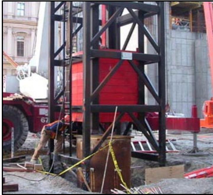
Figure 24-5, High-Strain Load Testing Apparatus (GRL Engineers, Inc. (2015))
